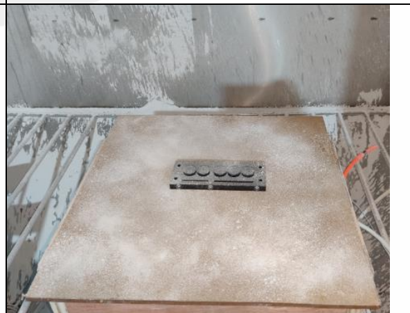
After IP5X test
