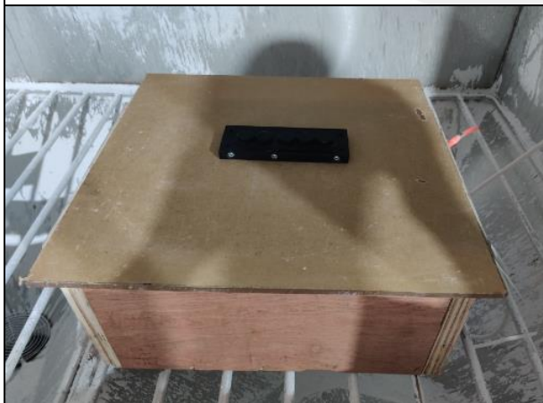
Before IP5X test
